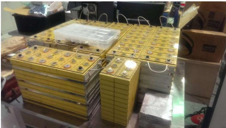
Figure 1 – Used 160Ah LiFePO4 Batteries
